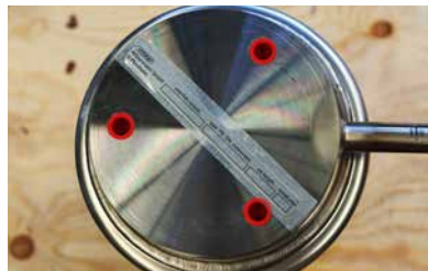
The expansion joints are fastened on a special retaining plate by means of three threaded blind holes
