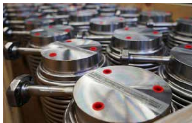
First delivery of the 750 flexible HYDRA® hydraulic expansion joints
