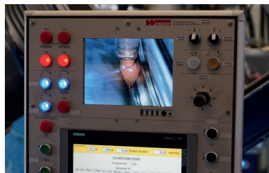
The bellows and tubular elements are monitored electronically and welded at a speed of 35 cm/min.
