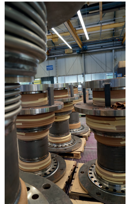
Before being packed into wooden boxes, the expansion joints with their protected bellows are standing in front of the painting line.
